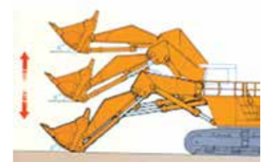
Auto Bucket level raise system
